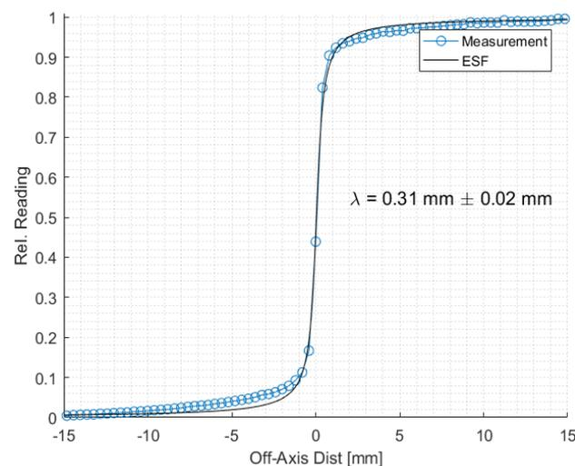
Figure 1: Measured signal produced by a lead block placed on the EPID. The fitted ESF is based on (2).
