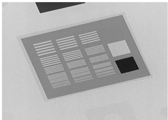
**Figure 5:** Deconvolved 1 MV portal image of the line
