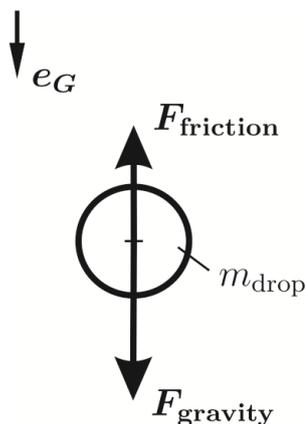
**Figure 1:** External forces acting on droplet in mid-air
