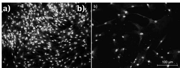
**Figure 2:** Cell nuclei on untreated (a) and modified DLC coatings (b).
