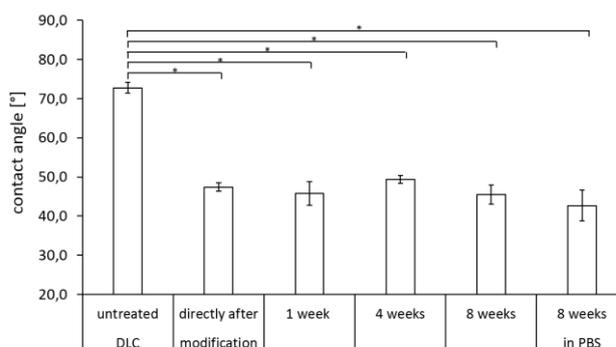
**Figure 3:** Contact angle on untreated and modified DLC during long-time storage under ambient conditions and in PBS.
