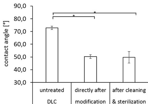
**Figure 1:** Contact angle on untreated and modified DLC and after cleaning and sterilization of the DLC surface.
