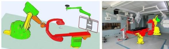
**Figure 1:** critical surfaces of the angiographic system (from red: very high to green: low)
