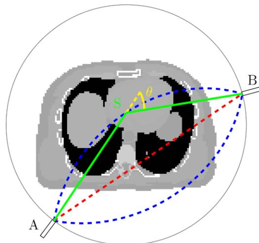
**Figure 1:** Visualization of one slice of the XCAT attenuation phantom and a PET scanner with two detectors in coincidence. Red dashed line: LOR of both detectors. Blue arcs: limits of the possible scatter locations for a given energy which is directly related to the scatter angle (highlighted in yellow). The emission must have occurred somewhere along the green lines and then scattered at one position of the upper arc inside the body contour.
