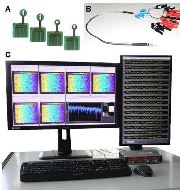
**Figure 1:** A) Different electrode designs with eight and sixteen channels B) An assembled electrode with connector cable C) Recording system consisting of a recording device and self-developed software showing sixteen time signals, six time-frequency plots and one spectrum.
