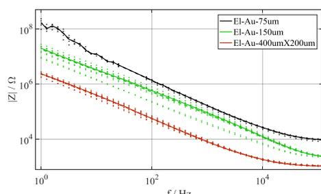
**Figure 3:** Measured magnitude of electrode impedances. Black:  $\varnothing$  75  $\mu\text{m}$ ; green:  $\varnothing$  150  $\mu\text{m}$ ; red: 400  $\mu\text{m}$  X 200  $\mu\text{m}$ . Dots representing single measurement points, lines represent calculated median value, dashed lines represent mean values.
