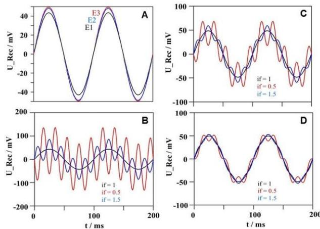
**Figure 5:** Simulation results; **A)** Dependency between electrode sizes (impedance) to the recorded signal. **B) – D)** Influence of impedance variances to the recorded signal, the capacitance CH2 was varied. In **B)** model values for E1, in **C)** model values for E2, and in **D)** model values for E3 were used.
