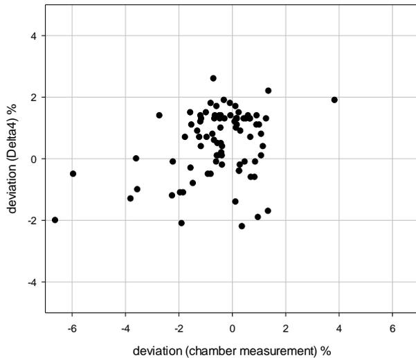
**Figure 2:** Deviation of Delta4 measurements vs measurements with the ionization chamber. For the Delta4 measurements the median dose deviation of all point with >60% of Dmax is used. Chamber measurements show the mean of 2 positions.
