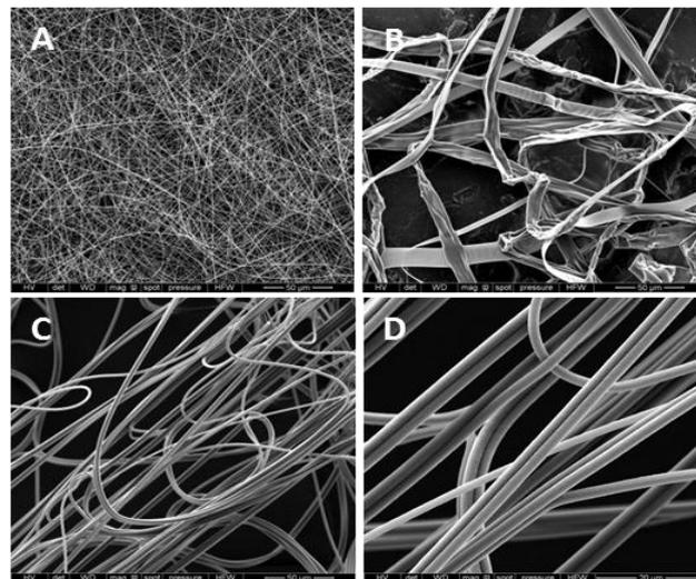
**Figure 1:** SEM images of the electrospun polyimide – Influence of the solvent on the shape of fibre (A: DMF (Entry 7b) smooth and round shaped fibres, B: HFIP (Entry 2) ribbon shaped fibres, C,D: DMSO (Entry 4) double attached fibres).
