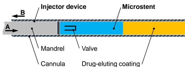
**Figure 2:** Schematic representation of the microstent loaded into the injector device for minimally invasive glaucoma surgery; Two alternative functional principles: a mandrel pushes the microstent out of the cannula (*A*) or the cannula is withdrawn above the microstent (*B*).
