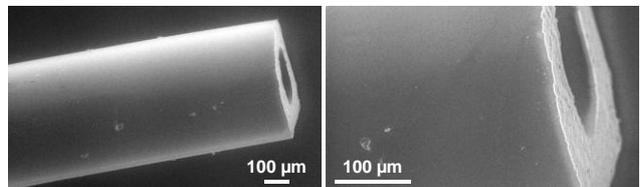
**Figure 4:** ESEM image of a simplified polymeric microstent: overview and detail of the outflow area (without drug-eluting coating).
