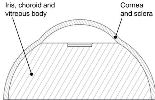
**Figure 3:** Simplified two-piece silicone eye model for applicability testing of injector devices.
