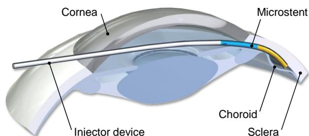
**Figure 1:** Concept of a microstent system for minimally invasive glaucoma surgery: valved inflow area of the microstent (blue) without and outflow area (orange) with drug-eluting coating.
