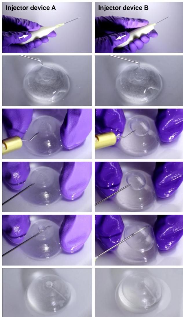
Figure 6: Microstent implantation into silicone eye model using the injector devices A and B; Top down: handling of the injector device, wetting of the silicone eye model, paracentesis, insertion of injector device into the anterior chamber, microstent implantation into suprachoroidal space and microstent localization after completion of the procedure.
