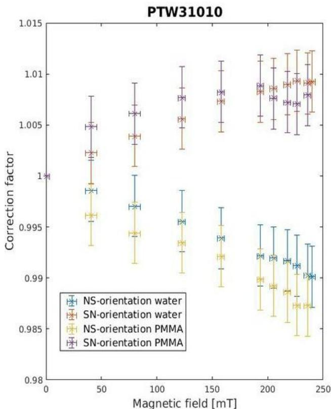
**Figure 2:** Correction factors for a PTW31010 ionization chamber for both magnetic field orientations, measured in PMMA and water.
