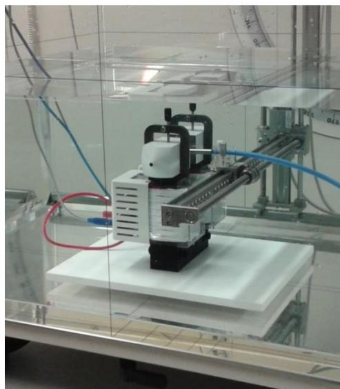
**Figure 1:** Experimental setup for the PTW31010 ionization chamber with electromagnet in the water phantom. Note that radiation beam direction is oriented from top to bottom, perpendicular to ionization chamber and magnetic field.
