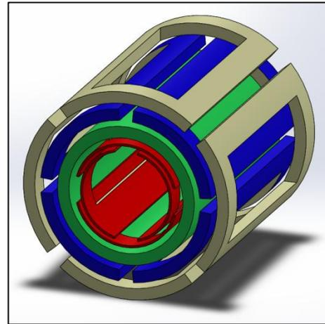
**Figure 3:** Coil topology of an electronically rotatable FFL Imaging-device. The red part represents the drive field coils for horizontal and vertical FFL translation, the green part the axial-gradient coil, the blue and the yellow part the quadrupoles.
