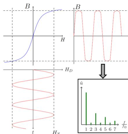
**Figure 1:** The basic principle of magnetic particle spectroscopy (MPS) and MPI. Applying an excitation field  $H_D$  with the fundamental frequency  $f_0$  causes a modulation of the magnetic flux density  $B(t)$  by the SPIONs. The receive signal  $u$ , which is proportional to the time derivative of  $B(t)$  then contains higher harmonics.
