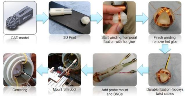
**Figure 5:** The process of the probe construction for the drive-field measurement. A mount head and a winding shape where printed by a photo-polymer 3D-printer, afterwards a 0.4 mm enamelled copper wire was wound around the shape and sealed with epoxy resin. After attaching BNCs, the probe was mounted onto the robot and driven into the measurement field.
