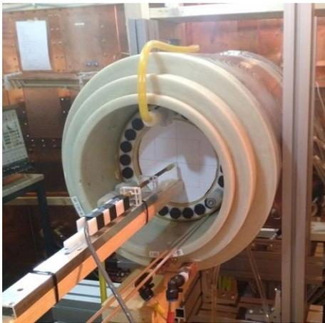
**Figure 4:** Setup of the selection-field measurement. A multi-axis hall-probe is mounted on a robot arm and records the magnetic flux density at various positions inside the bore.
