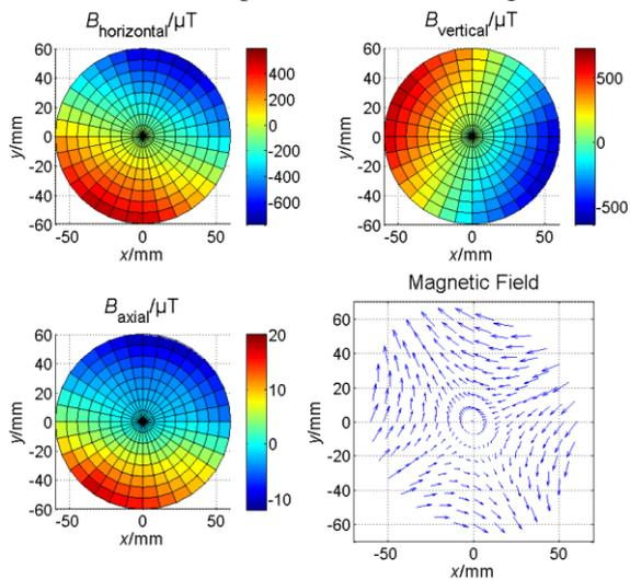
**Figure 6:** Interpolated magnetic flux density based on the Measurement in section 2.2. The top row shows the radial field components  $B_{\text{horizontal}}$  and  $B_{\text{vertical}}$ , the bottom row the axial field component  $B_{\text{axial}}$  and the field direction and relative magnitude.
