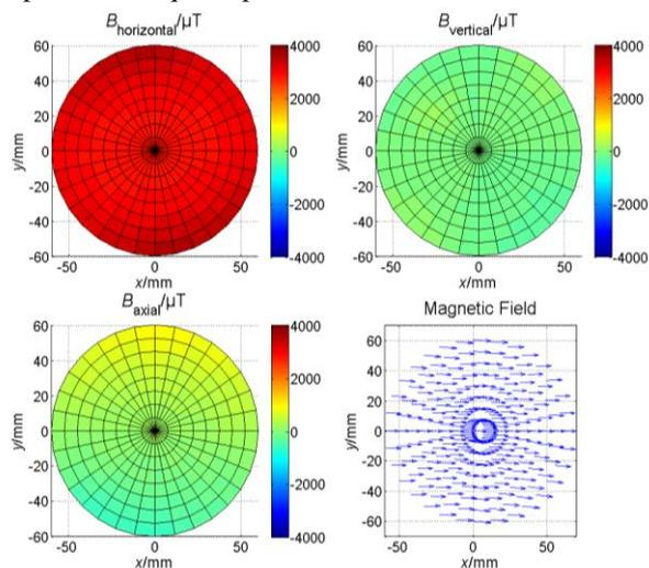
**Figure 7:** Interpolated magnetic flux density of the horizontal drive-field coil on a slice at the center of the bore.
