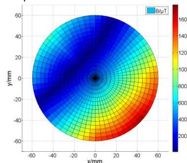
**Figure 9:** Rotated and translated FFL. In this simulated point in time, the FFL is rotated by 45° and translated by 15 mm.
