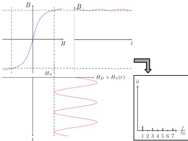
**Figure 2:** For spatial encoding, a selection field  $H_s$  is added, that shifts all SPIONs within the measurement field that are not in the close vicinity of the FFP or the FFL into magnetic saturation. Those particles do not respond to the drive field  $H_D$ .
