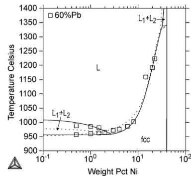
**Figure 5.** Calculated liquidus temperatures of Cu–Ni–Pb alloys at low nickel contents, together with experimental data points [15]. Solid lines refer to the calculations of this study and dashed lines refer to those of [24].
