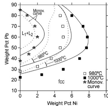
**Figure 4.** Calculated liquidus surfaces of the Cu–Ni–Pb system (a) and an enlarged section from the Cu–Pb side, together with experimental data points [13–16]. In Fig. 4b, the experimental data points are from the smoothed experimental data of Pelzel [15]. Solid lines refer to the calculations of this study and dashed lines refer to those of [24].
