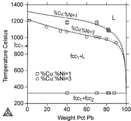
**Figure 7.** Calculated isopleths of the Cu–Ni–Pb system at composition ratios of wt% Cu / wt% Ni = 1 and wt% Cu / wt% Ni = 3, together with experimental data points [14,15]. Solid lines refer to the calculations of this study and dashed lines refer to those of [15].
