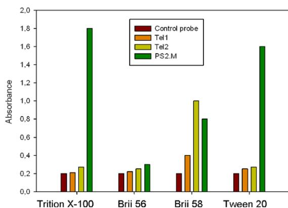
**Figure 3.** Comparison of absorbances at 417 nm obtained for indicator ABTS reaction catalyzed by DNAzymes in the presence of different surfactants.
