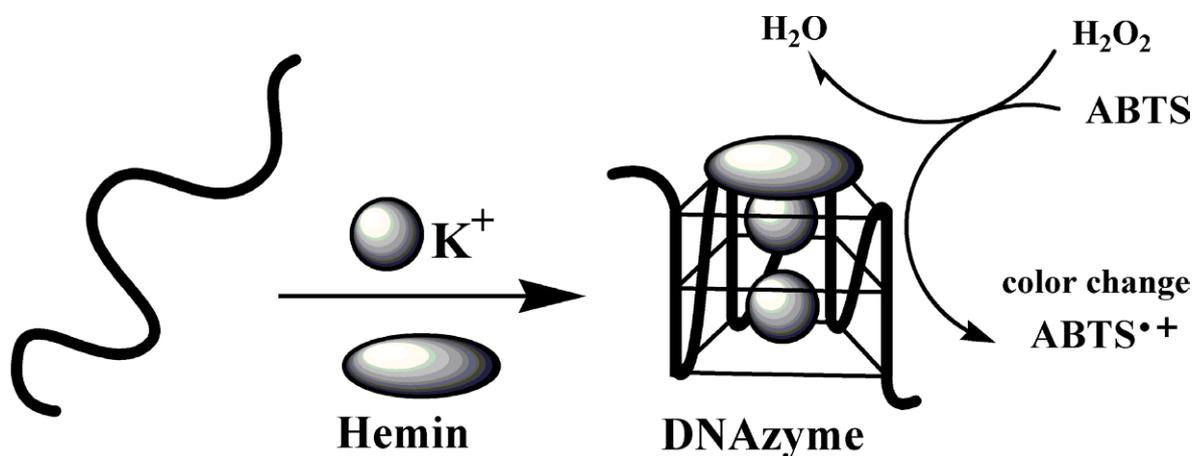
**Figure 1.** Schematic representation of the DNAzyme based on the G-quadruplex of telomeric repeat sequence and the indicator reaction with ABTS.
