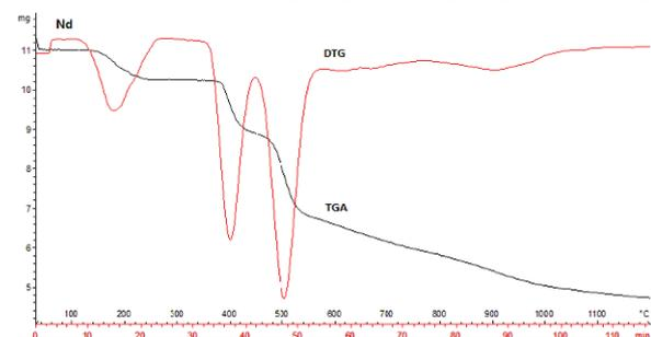
**Figure 5.** TGA-DTG curves showing the decomposition of  $[\text{Gd}_2(\text{NIC})_6(\text{H}_2\text{O})_4]$  and  $[\text{Nd}_2(\text{NIC})_6(\text{H}_2\text{O})_4]$  at a heating rate of 10  $\text{K min}^{-1}$  in a nitrogen atmosphere.
