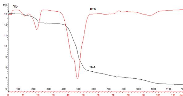
**Figure 4.** TGA-DTG curves showing the decomposition of  $[\text{Yb}_2(\text{NIC})_6(\text{H}_2\text{O})_4]$  at a heating rate of 10 ( $\text{K min}^{-1}$ ) in a nitrogen atmosphere.
