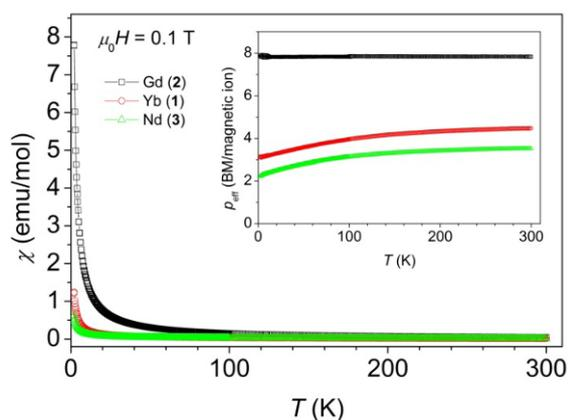
**Figure 6.** Molar susceptibility as a function of temperature measured in a magnetic field of 0.1 T. Inset shows an effective magnetic moment as a function of temperature calculated per magnetic ion.
