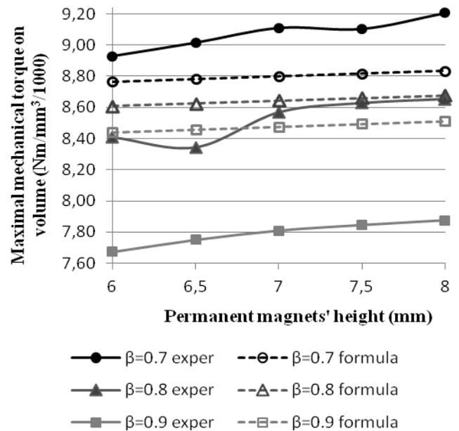
Fig. 6. The function  $M_{max}=f(h, \beta)$  ( $l = 30$  mm).
