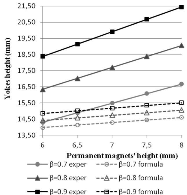
Fig. 7. The function  $h_{yoke}=f(h, \beta)$  ( $l = 30$  mm).
