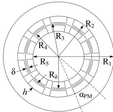
Fig. 1. Dimensions of cylindrical magnetic coupler in a cross-section.  $R_1$ - $R_5$  – radiuses;  $R_{\delta}$  – radius of air gap's middle circle;  $\delta$  – air gap;  $h$  – PMs height;  $\alpha_{PM}$  – angle of PM.
