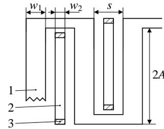
Fig. 3. The fragment of the topology of meander slow-wave system with additional shields grounded at both edges, where  $2A = 20$  mm;  $w_1 = 0.5$  mm;  $w_2 = 0.25$  mm;  $s = 0.65$  mm;  $\epsilon_r = 7.3$ ;  $h = 0.5$  mm.
