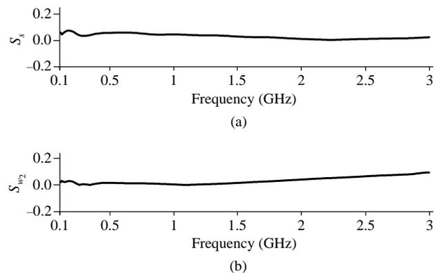
Fig. 6. Impact coefficients on the phase delay time of a system when changing: (a) the gap  $s$  between adjacent meander conductors; (b) the width  $w_2$  of additional shield.
