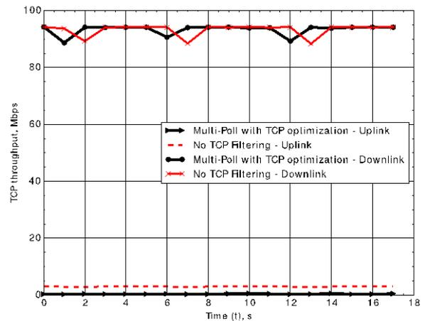
Fig. 11. Comparison of uplink and downlink when TCP filtering was turned off and on.
