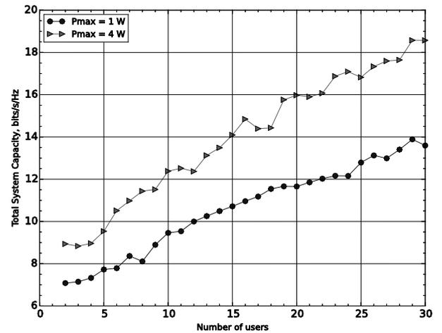
Fig. 2. Total system capacity with 30 users in the system with different allowed power levels.
