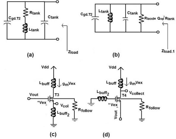
**Figure 2.** a) The load impedance network formed by the resonance tank; b) an equivalent model showing the effect of tank resistance on output load impedance; c) alternative source-follower output buffer; d) common-gate output buffer
