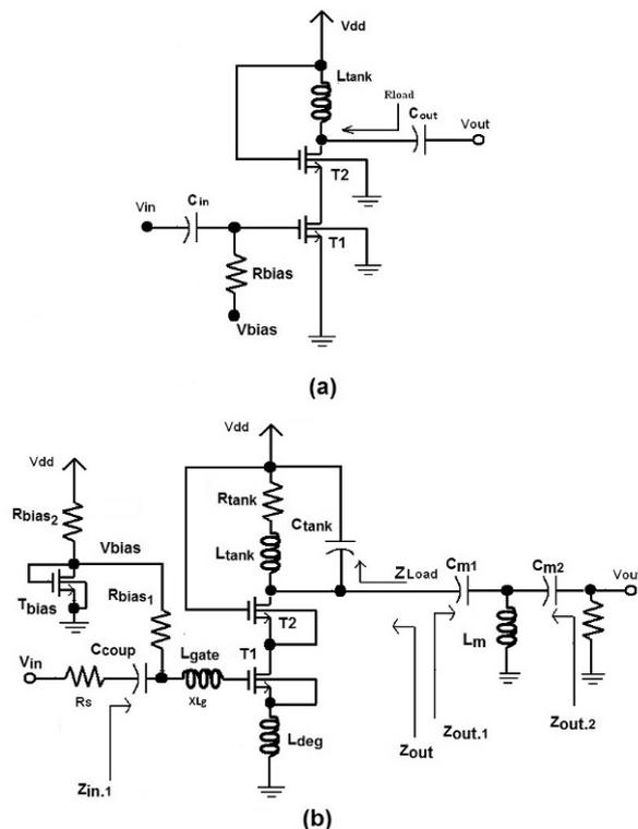
**Figure 1.** a) The basic common source unmatched (core) stacked amplifier; b) the proposed K-band single-stage matched wideband amplifier with a diode-connected biasing device
