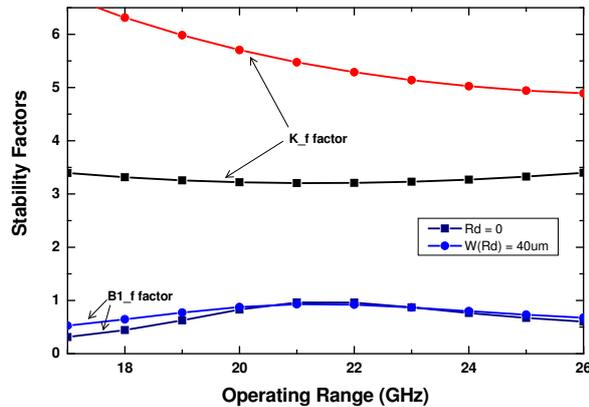
**Figure 8.** Upward shift in the Rollette stability factors ( $K_f$  and  $B_{1f}$ )
