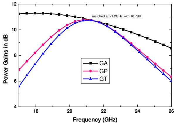
Figure 4. Power gains for the amplifier core and the matched LNA (without regulation).
