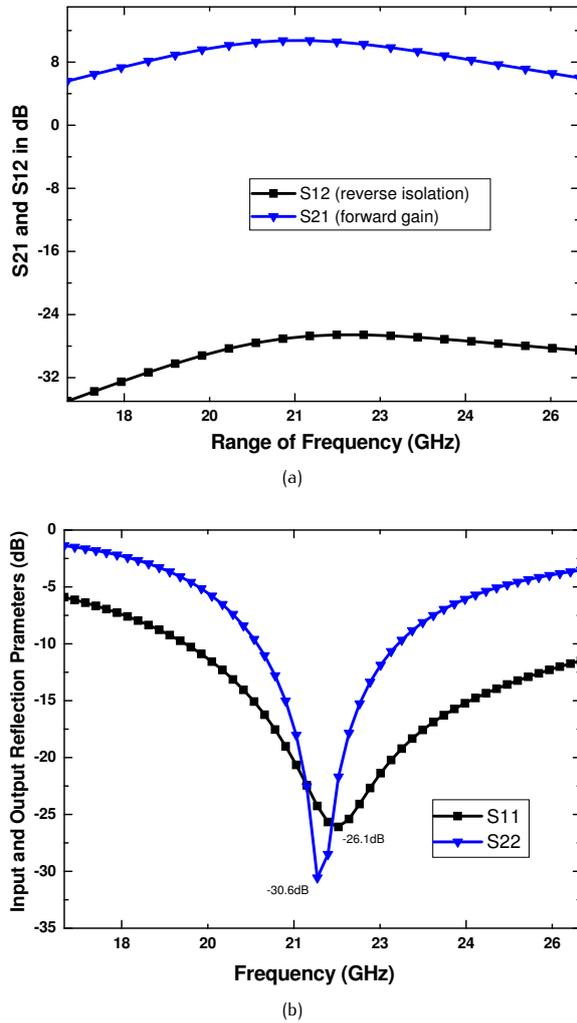
Figure 3. a) Forward gain ( $S_{21}$ ) and reverse isolation ( $S_{12}$ ) figures; b) port reflection parameters (for the unregulated amplifier).
