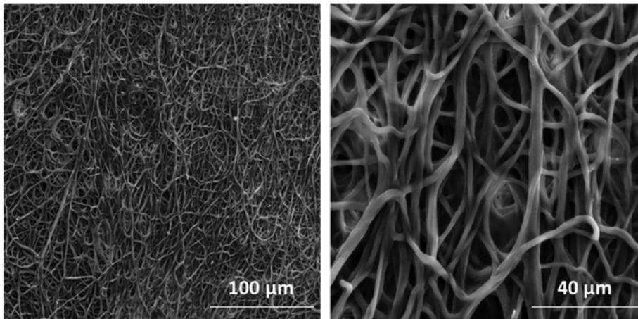
Figure 3: SEM images of PLA/PCL40 membrane, polylactide nanofibers side.
