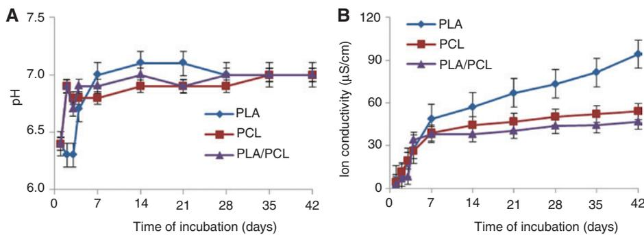
**Figure 8:** pH (A) and ion conductivity (B) changes during 6 weeks of incubation in distilled water.
