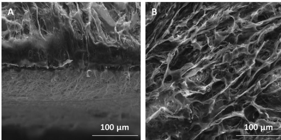
Figure 4: SEM images of PLA/PCL40 membrane: the cross-section (A) and PCL side (B).
