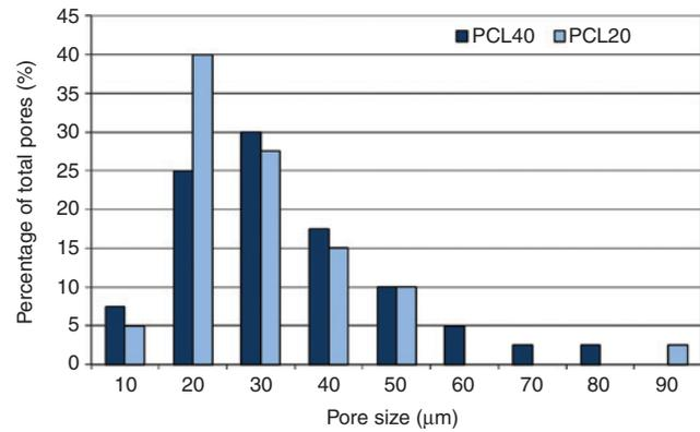
**Figure 2:** Average pore size distribution comparing PCL20 and PCL40.
