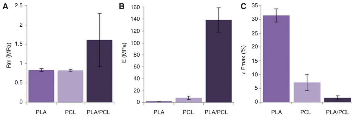
**Figure 7:** Tensile strength  $R_m$  (A), Young's modulus  $E$  (B) and maximum elongation  $\epsilon_{Fmax}$  (C) of studied membranes.
