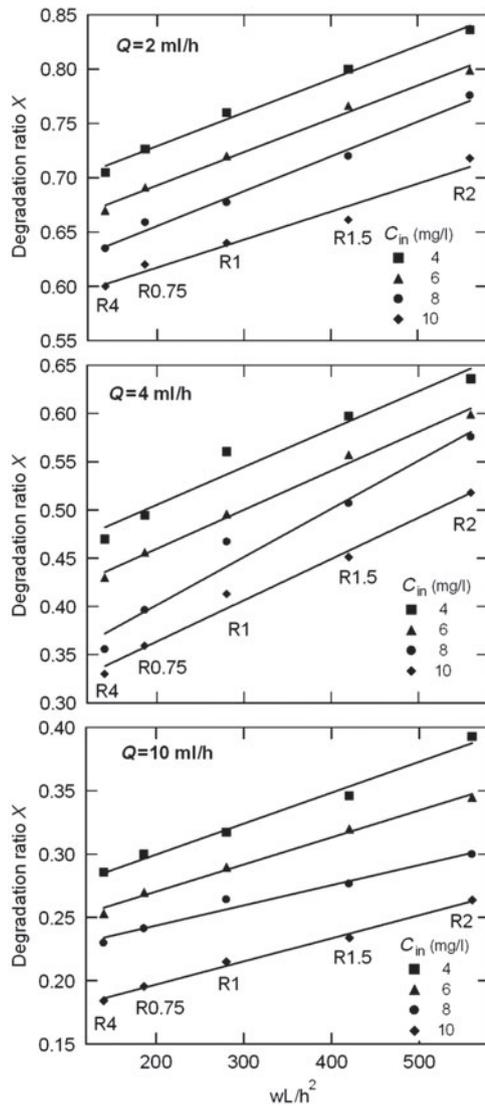
**Figure 6** Degradation of salicylic acid as a function of the dimensions of the microchannel reactors ( $wL/h^2$ ) for different inlet concentrations ( $C_{in}$ ) and flow rates ( $Q$ ).  $w$  refers to the channel width,  $L$  to the channel length, and  $h$  to the channel height. The lines represent the best linear fits given by  $X=a(wL/h^2)$ .
