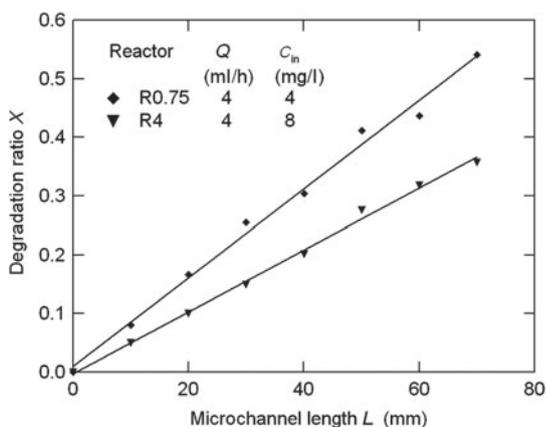
**Figure 5** Degradation ratio ( $X$ ) of salicylic acid as a function of the microchannel length ( $L$ ) for different inlet concentrations ( $C_{\text{in}}$ ) and polymeric reactors. The reactors used are similar in width and height to R0.75 ( $w=1.5$  mm and  $h=0.75$  mm) and R4 ( $w=2$  mm and  $h=1$  mm). The lines represent the best linear fits given by  $X=0.0076 L + 0.0097$  ( $R^2=0.992$ ) for R0.75, and  $X=0.0053 L - 0.0026$  ( $R^2=0.996$ ) for R4.
