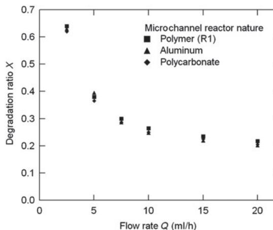
**Figure 3** Degradation of salicylic acid in the polymeric, aluminum, and polycarbonate microchannel reactors as a function of the flow rate. Geometrical characteristics of the reactors:  $w=1$  mm,  $h=0.5$  mm, and  $L=70$  mm. Experimental conditions:  $C_{in}=10$  mg/l and  $I=1.5$  mW/cm<sup>2</sup>.
