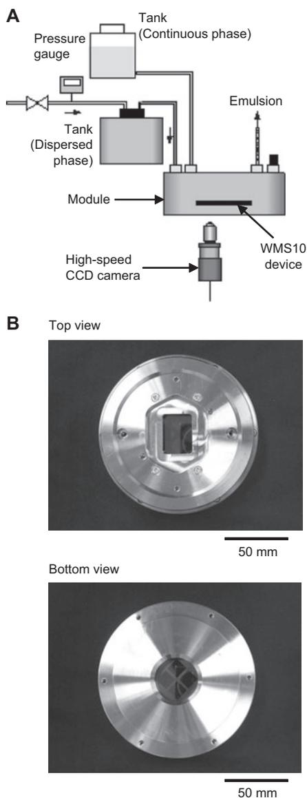
**Figure 3** (A) Simplified schematic drawing of the large MC emulsification device developed in this study. (B) Top and bottom views of the module.
