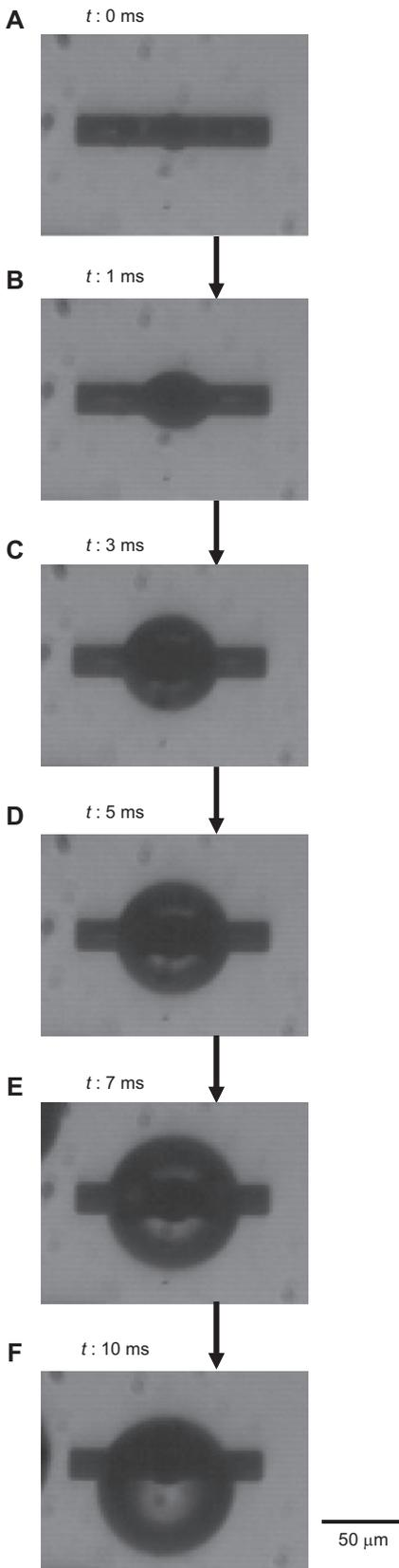
**Figure 4** Sequential micrographs of the droplet detachment process from a slot outlet.  $t$  denotes time. The continuous phase flows from top to bottom in the micrographs.
