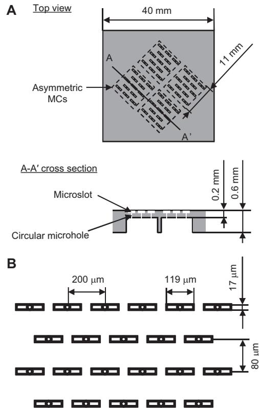
**Figure 2** (A) Schematic representation of the WMS10 chip. (B) Schematic diagram of asymmetric MCs on the top side of the plate.
