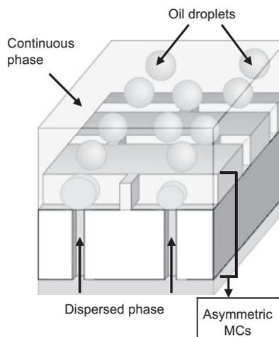
**Figure 1** Three-dimensional schematic drawing of the generation of O/W emulsion droplets via asymmetric MCs.
