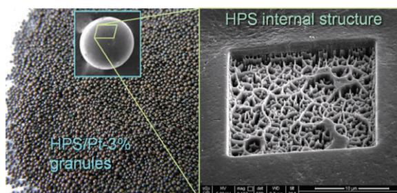
**Figure 1** The structure of HPS-based Pt catalyst. Left: HPS/Pt 3% granules; right: the internal HPS structure imaged by scanning electron microscopy.
