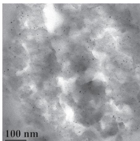
**Figure 2** TEM of HPS-stabilized Pd NPs.
