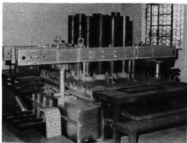
Fig. 4: Mg electrolytic cell.
