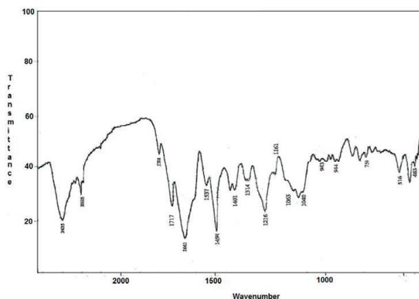
**Figure 4.** FTIR spectrum in unit  $\text{cm}^{-1}$  of PAI-nanocomposite films **5a**.
