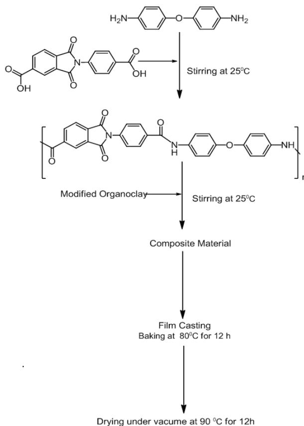
**Figure 3.** Flow sheet diagram for the synthesis of PAI-nanocomposites film **5a** and **5b**.
