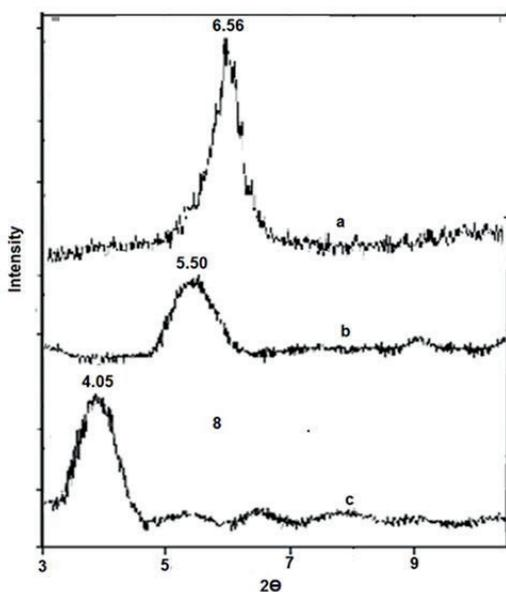
**Figure 5.** X-ray diffraction patterns of Organoclay (**a**), PAI-nanocomposite films **5a** (**b**) and **5b** (**c**).
