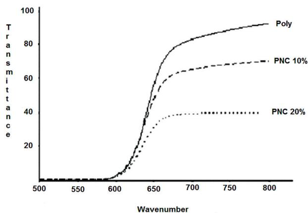
**Figure 7.** UV-vis spectra in unit of  $\text{cm}^{-1}$  of PAI **5**, PAI-nanocomposite films **5a** and **5b**.
