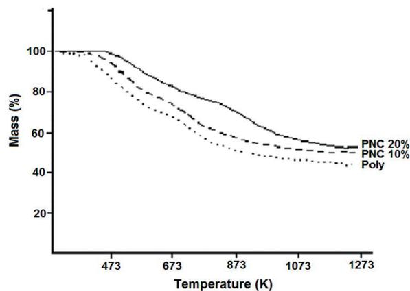
**Figure 8.** TGA thermograms of neat PAI **5** and PAI-nanocomposite films **5a** and **5b**.
