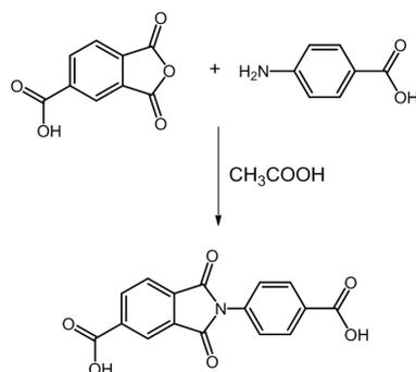
**Figure 1.** Synthetic route of *N*-trimellitimidido-4-amino benzoic acid **3**.
