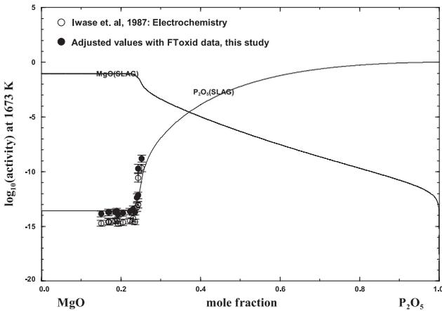
**Fig. 5:** Calculated activity of P<sub>2</sub>O<sub>5</sub>(l) in the MgO-P<sub>2</sub>O<sub>5</sub> system along with experimental data [42]. The Gibbs energy of pure liquid P<sub>2</sub>O<sub>5</sub> of Iwase et al. [42] was corrected according to the new P<sub>2</sub>O<sub>5</sub> Gibbs energy by Jung and Hudon [3] to ensure a thermodynamically consistent database development.
