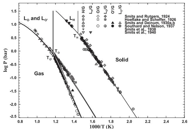
**Fig. 1:** Log P vs 1000/T diagram of the P<sub>2</sub>O<sub>5</sub> unary used in the present study. O'-P<sub>2</sub>O<sub>5</sub> is the most stable solid phase and melts at 580°C. Details of the thermodynamic modeling results can be found in reference [2].
