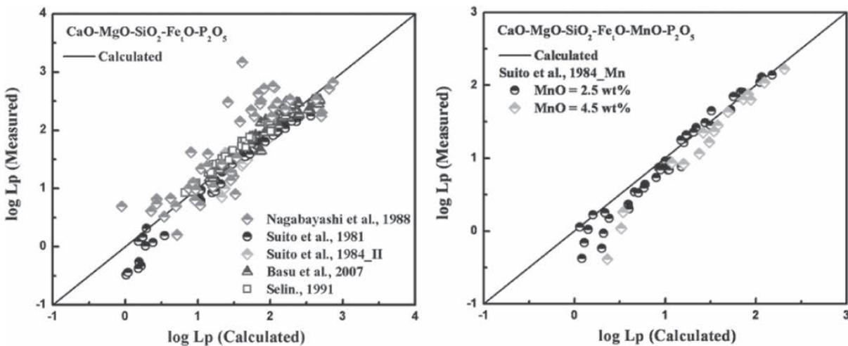
Fig. 9: Comparison between experimental and calculated  $L_p$  values for the  $\text{CaO-MgO-SiO}_2\text{-Fe}_1\text{O(-MnO)}$  system [51–53, 60–61, 69–70].
