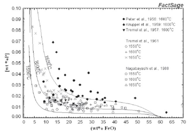
**Fig. 6:** (a) The calculated phase diagram of the CaO-Fe<sub>1</sub>O-P<sub>2</sub>O<sub>5</sub> system equilibrated with molten Fe at 1600°C, (b)  $L_p$  between molten iron and the slag along CaO saturation line, and (c) the relationship between [%P] in liquid Fe and Fe<sub>1</sub>O content in slag along CaO saturation line in comparison with available experimental data [16, 45–51].
