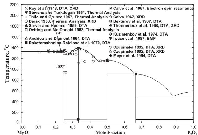
**Fig. 4:** Optimized binary phase diagram of the MgO-P<sub>2</sub>O<sub>5</sub> system with experimental data [20, 29–44].
