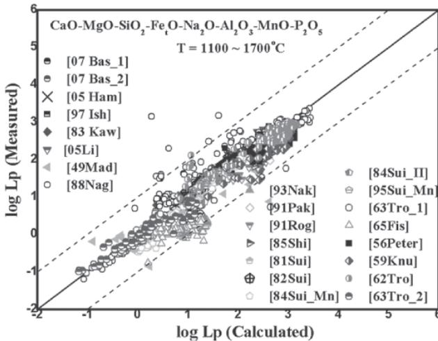
Fig. 8: Comparison between experimental [16, 45, 47, 51–70] and calculated  $L_p$  values for binary, ternary and multicomponent slags using the present thermodynamic database.
