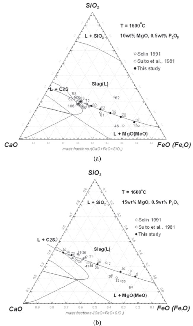
**Fig. 7:** Calculated phosphorus distribution between slag and molten Fe for the  $CaO-Fe_1O-SiO_2-MgO$  slag at  $1600^\circ C$  in comparison with experimental data [52–53]. (a)  $CaO-Fe_1O-SiO_2-10\%$   $MgO$  slag and (b)  $CaO-Fe_1O-SiO_2-15\%$   $MgO$  slag. Upright numbers in the diagram are experimental  $L_p$  data and underlined numbers are the calculated  $L_p$  values from the present database.
