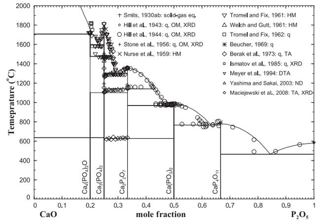
**Fig. 2:** Optimized binary phase diagram of the CaO-P<sub>2</sub>O<sub>5</sub> system with experimental data [8–22].
