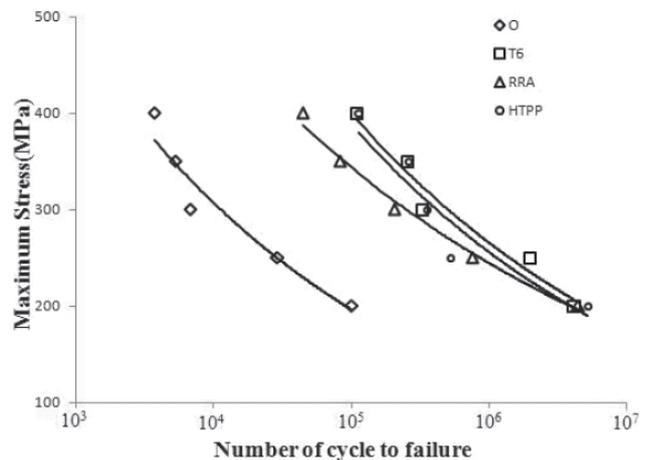
Fig. 6: S – N diagram obtained at the end of fatigue tests of the AA7075 aluminum alloy aged through O, T6, RRA and HTPP heat treatment processes
