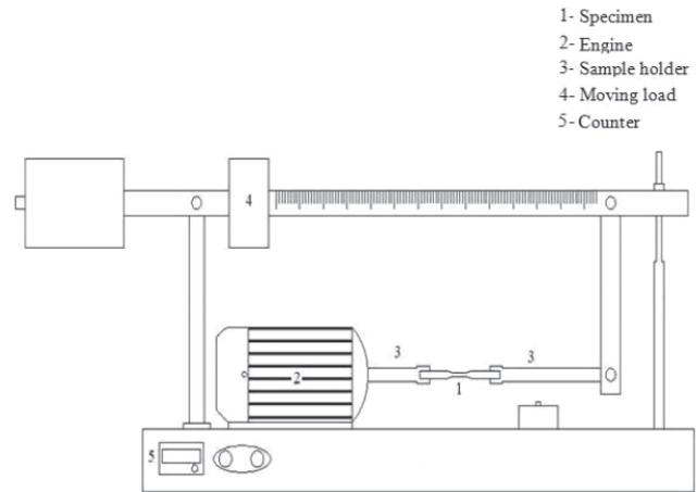
Fig. 2: Schematic image of the rotary tilt fatigue test device
