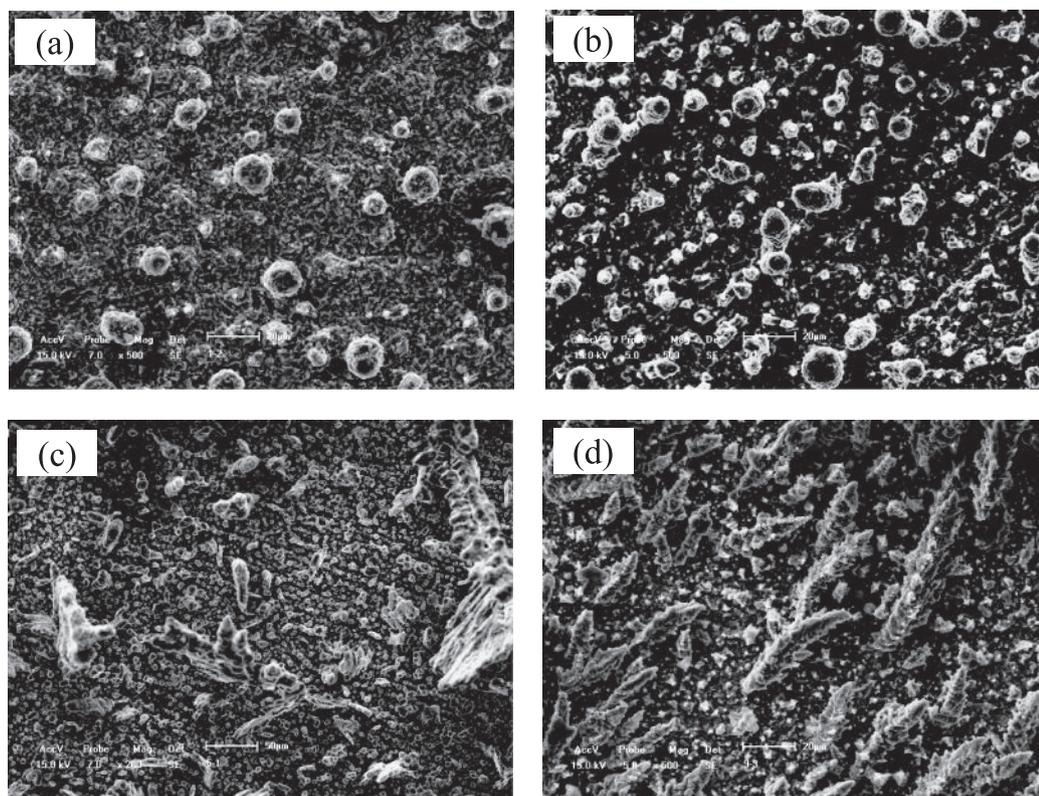
**Fig. 4:** SEM micrographs of aluminum electrodeposits prepared on Cu electrodes in 1.3:1 molar ratio  $\text{AlCl}_3$ - $\text{NaCl}$  molten salts using  $25 \text{ mA}\cdot\text{cm}^{-2}$  current density at  $170^\circ\text{C}$  for different electrolysis time. The electrolysis time is 0.5 h (a), 1 h (b), 1.5 h (c) and 2 h (d) respectively.
