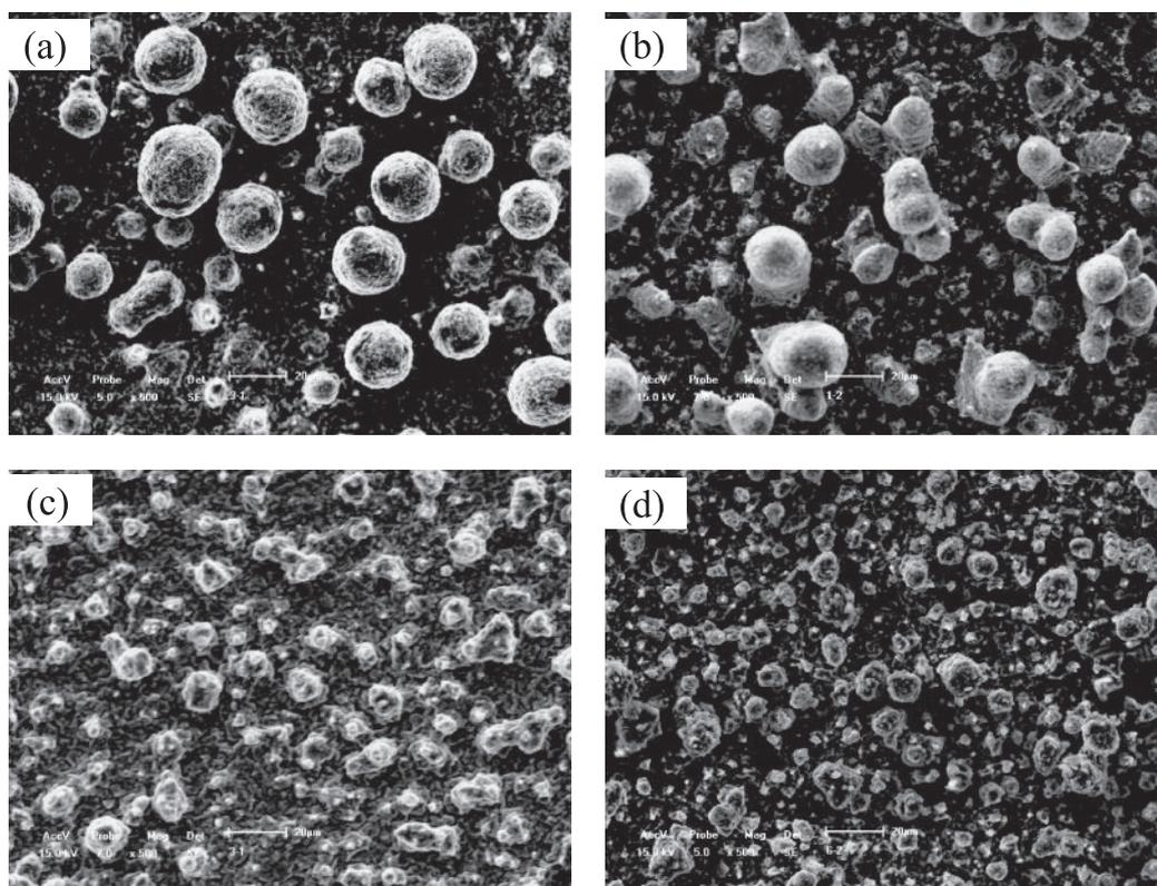
**Fig. 3:** SEM micrographs of aluminum electrodeposits prepared on Cu electrodes in different molar ratio  $\text{AlCl}_3$ - $\text{NaCl}$  molten salts at constant current density  $50 \text{ mA}\cdot\text{cm}^{-2}$  for 0.5 h at  $170^\circ\text{C}$ . (a)  $n_{\text{AlCl}_3}/n_{\text{NaCl}} = 1.3$ ; (b)  $n_{\text{AlCl}_3}/n_{\text{NaCl}} = 1.5$ ; (c)  $n_{\text{AlCl}_3}/n_{\text{NaCl}} = 1.7$ ; (d)  $n_{\text{AlCl}_3}/n_{\text{NaCl}} = 1.9$ .
