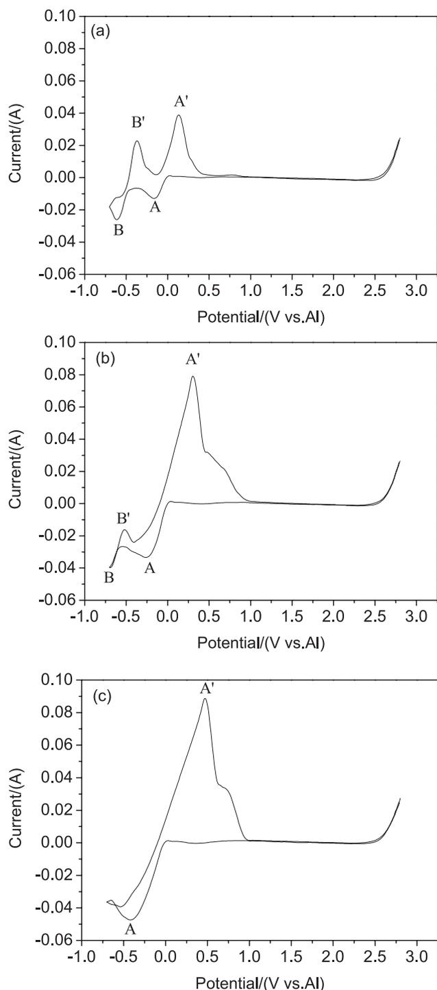
**Fig. 1:** Cyclic voltammograms recorded on W electrode in different molar ratio  $\text{AlCl}_3$ -NaCl molten salts at  $170^\circ\text{C}$ . Scan rates:  $0.1\text{ V/s}$ . (a)  $n_{\text{AlCl}_3}/n_{\text{NaCl}} = 1.1$ ; (b)  $n_{\text{AlCl}_3}/n_{\text{NaCl}} = 1.3$ ; (c)  $n_{\text{AlCl}_3}/n_{\text{NaCl}} = 1.5$ .
