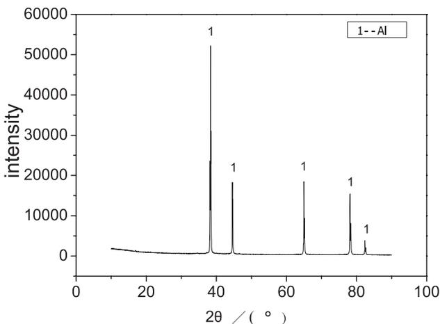
**Fig. 5:** X-ray diffraction pattern of aluminum deposit
