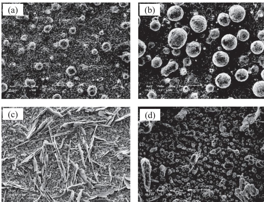
**Fig. 2:** SEM micrographs of aluminum electrodeposits prepared on Cu electrodes from 1.3:1 molar ratio AlCl<sub>3</sub>-NaCl molten salts at 170°C for 0.5 h. The applied current densities are 25 mA·cm<sup>-2</sup> (a), 50 mA·cm<sup>-2</sup> (b), 75 mA·cm<sup>-2</sup> (c) and 100 mA·cm<sup>-2</sup> (d) respectively.
