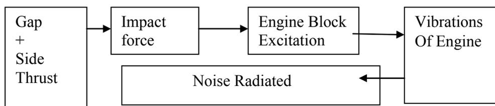
Fig.1. Generation of Piston Slap Noise.
