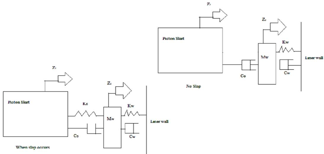
Fig.7. Lumped impact model.
