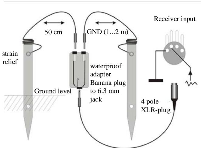
Fig. 5. Self-made ground spikes to use as ELF-sensors
