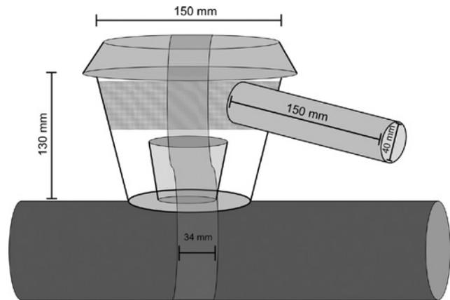
**Figure 1:** Schematic representation of round-pot feeder placed on a tree branch.
