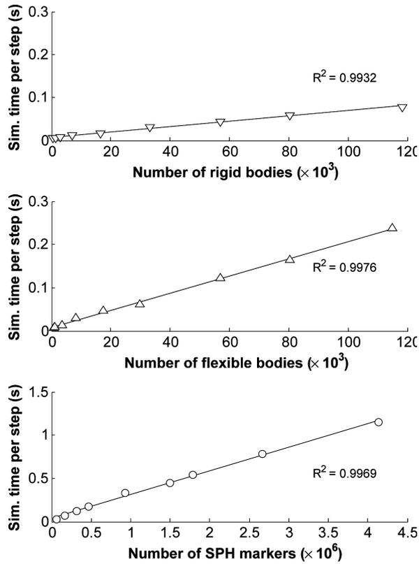
Fig. 5. Scaling analysis of Chrono::Fluid for rigid body dynamics, flexible body dynamics, and fluid dynamics as function of problem size ( $N_r$ ,  $N_f$ , and  $N_m$ , respectively). The coefficients  $R^2$  are specified to each linear regression
