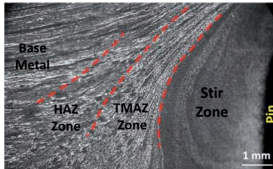
Fig. 7. The macro-structure of the plunge section (conducted at rotation speed 800 RPM)
