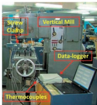
Fig. 3. Welding equipment and temperature measurement instruments
