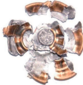
Fig. 6. Projectile deformation in the final stage – experimental result
