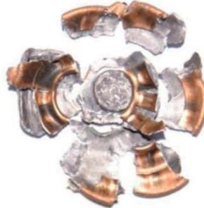
Fig. 6. Projectile deformation in the final stage – experimental result
