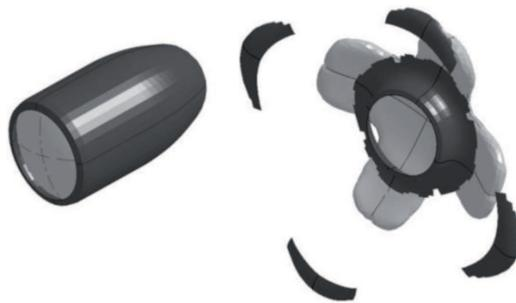
Fig. 5. Projectile deformation in the final stage – numerical result
