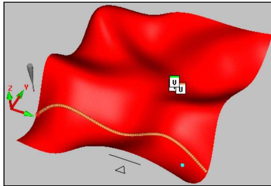
Fig. 2. The location of the scanned section on the CAD model ( $U, V$  – directions of the surface parameterization, PC DMIS software)
