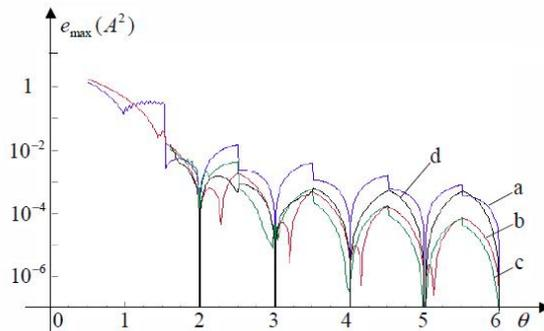
Fig. 4. Maximal relative values of errors of the amplitude power estimation with the multi-point DFT interpolations for the Hann window ( $\theta$  is obtained with the three-point interpolation (18)): a – the one-point est. (21), b – the three-point est. (23), c – the five-point est. (24), d – the five-point EBM est. (11).
