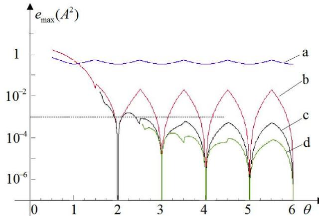
Fig. 2. Maximal relative values of errors of the amplitude square estimation by (11) and the Hann window: a – the one-point est. ( $r=0$ ), b – the three-point est. ( $r=1$ ), c – the five-point est. ( $r_{\text{optimal}}=2$ ), d – the seven-point est. ( $r=3$ ).
