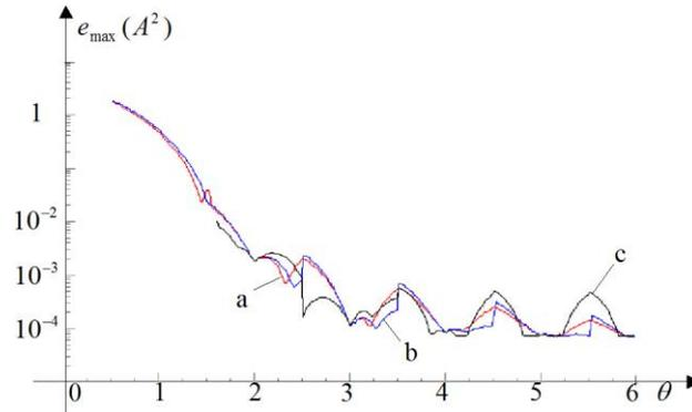
Fig. 10. Maximal relative values of errors of the amplitude square estimation in experiment using the Hann window ( $\theta$  is obtained with the three-point interpolation (18)): a – the IDFT est. (23), b – the squared DFT est. (39), c – the five-point EBM est. (11).
