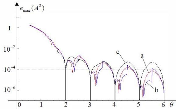
Fig. 6. Maximal relative values of errors of the amplitude square estimation with the three-point DFT interpolations for the Hann window ( $\theta$  is obtained with the three-point interpolation (18): a – the IDFT est. (23), b – the squared DFT est. (39), c – the five-point EBM est. (11).
