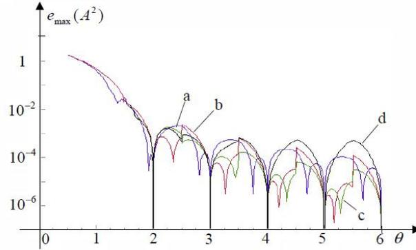
Fig. 5. Maximal relative values of errors of the amplitude square estimation with the multi-point DFT interpolations for the Hann window ( $\theta$  is obtained with the three-point interpolation (18): a – the two-point est. (32), b – the three-point est. (39), c – the five-point est. (40), d – the five-point EBM est. (11).
