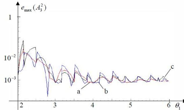
Fig. 11. Maximal relative values of errors of the squared amplitude of the third component in experiment using the triangular shape signal ( $\theta$  is obtained with the three-point interpolation (18)): a – the IDFT est. (23), b – the squared DFT est. (39), c – the five-point EBM est. (11).
