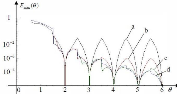
Fig. 3. Maximal absolute values of errors of the relative frequency estimation with the multi-point DFT interpolations for the Hann window: a – the three-point EBM est. (19)  $r = 1$ , b – the five-point EBM est. (19)  $r_{optimal} = 2$ , c – the seven-point EBM est. (19)  $r = 3$ , d - the three-point DFT interpolation (18).
