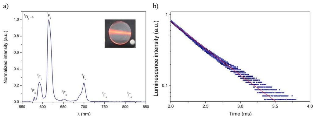
Fig. 1. a) The luminescence spectrum of PMMA doped with trivalent europium compounds at exc. 355 nm with observed transitions (all the transitions start from the  ${}^5\text{D}_0$  state); b) The luminescence decay time measurement results (at 616 nm).
