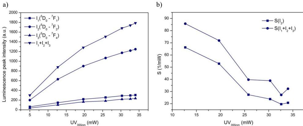
Fig. 5. a) The maximum peak intensity for sensor A at exc. 355 nm; b) the calculated sensitivity.
