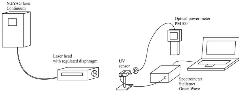
Fig. 3. A scheme of the measurement setup.
