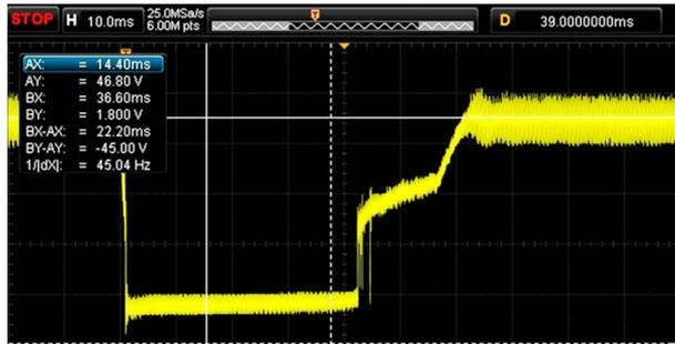
Fig. 12. The response to a short load pulse for a system consisting of larger solar panels.
