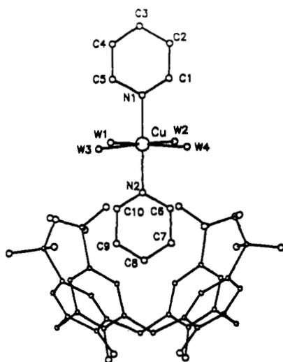
Fig. 3.  $[\text{Cu}(\text{NC}_5\text{H}_5)_2(\text{H}_2\text{O})_4]^{2+}$  as a guest in  $[\textit{p}\text{-sulfonatocalix[4]arene}]^{5-}$ .
