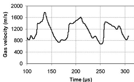
Fig. 3 Predicted time-evolution of gas velocity at the torch exit on torch axis.  $D_{\text{nozzle i.d.}} = 7 \text{ mm}$ ;  $I = 300 \text{ A}$ .
