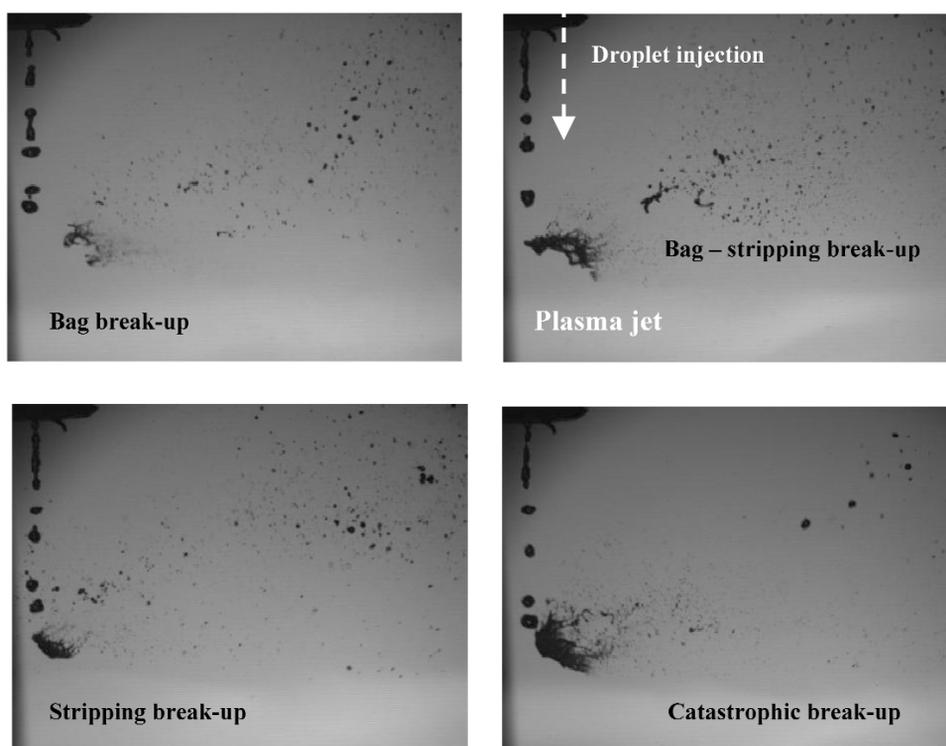
**Fig. 7** Photographs of 250- $\mu\text{m}$ -diameter water drops penetrating the transverse plasma jet. Various break-up regimes are observed depending on the time when the drops penetrate the gas flow. Torch nozzle exit diameter: 7 mm; arc current: 600 A; gas flow rate: 45 Nl/min Ar +15 Nl/min H<sub>2</sub>.
