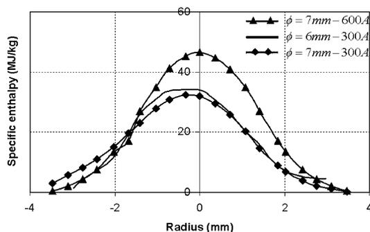
Fig. 5 Predicted time-averaged radial profile of gas specific enthalpy at nozzle exit.
