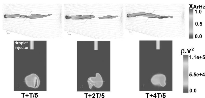
**Fig. 6** Time-evolution of the 5000-K isotherm colored by the mass fraction of plasma gas and of the gas momentum density ( $\text{kg} \cdot \text{m}^{-1} \cdot \text{s}^{-2}$ ) in the droplet injection plane.  $T$  is the arc fluctuation period. Ar (45 NL/min);  $\text{H}_2$  (15 NL/min); arc current: 600 A; torch nozzle diameter: 6 mm .
