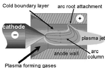
**Fig. 1** Schematic representation of a non-transferred DC plasma torch [25].
