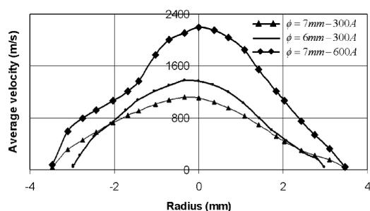
Fig. 4 Predicted time-averaged radial profile of gas velocity at nozzle exit;  $D_{\text{nozzle i.d.}} = 7 \text{ mm}$ ;  $I = 300 \text{ A}$ , 45 NI/min Ar +15 NI/min/  $\text{H}_2$ .
