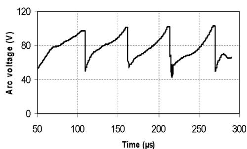
Fig. 2 Predicted time-evolution of the arc voltage.  $D_{\text{nozzle i.d.}} = 7 \text{ mm}$ ;  $I = 300 \text{ A}$ , 45 NI/min Ar +15 NI/min/  $\text{H}_2$ .
