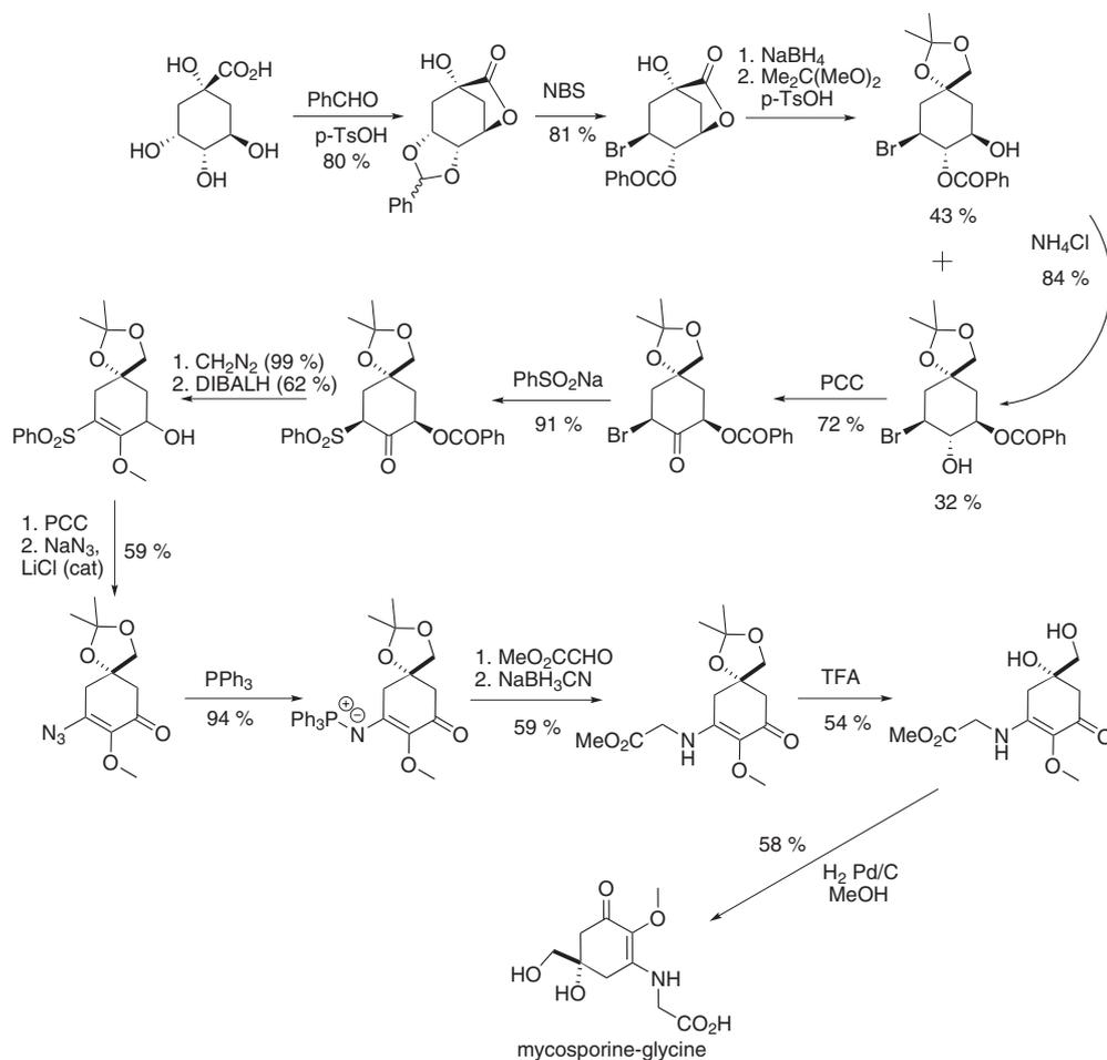
Fig. 10: Scheme of direct synthetic pathway described in 1995 [66].
