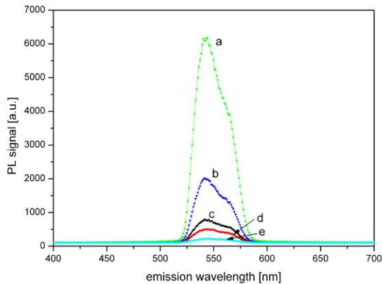
**Figure 1.** Spectrally resolved PL signal for LiF detectors irradiated with alpha particles (a –  $1.2 \times 10^{10} \text{ cm}^{-2}$ , b –  $1.7 \times 10^9 \text{ cm}^{-2}$ ) and gamma rays (c – 180Gy, d – 5Gy) during stimulation with a blue light (433 nm) with an application of two filters 550FIR25 (Knight Optical) and GG495 (Schott) at the emission. Curve e represents the background level.
