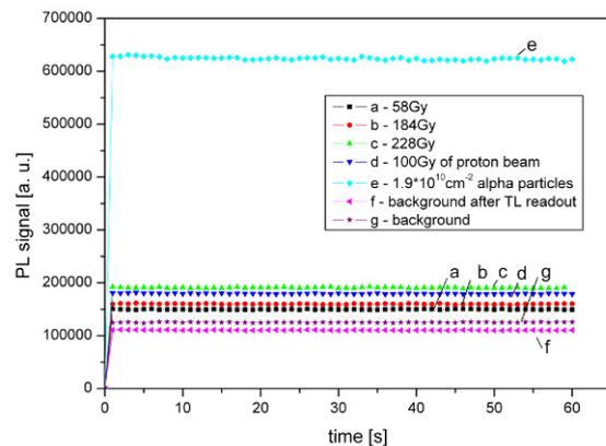
**Figure 3.** PL signal for LiF detectors irradiated with 58Gy, 184Gy and 228Gy of Cs-137 gamma rays, alpha particles with a fluence of  $1.9 \times 10^{10} \text{ cm}^{-2}$  of Am-241 source and 100Gy of 60MeV protons beam.
