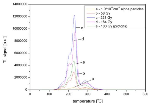
**Figure 4.** TL signal for LiF detectors irradiated with 58 Gy, 184 Gy and 228 Gy of Cs-137 gamma rays, alpha particles with a fluence of  $1.9 \times 10^{10} \text{ cm}^{-2}$  of Am-241 source and 100 Gy of 60 MeV protons beam.
