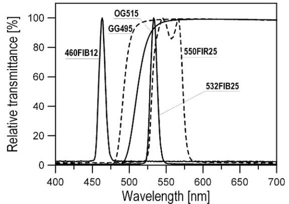
**Figure 2.** Relative transmittance characteristics of optical filters. Dashed lines represent 550FIR25 and GG495 filters, which were used for measuring PL emission (Fig. 1). The other filters, represented by solid lines, were used in PL reader: 460FIB12 for excitation and 532FIB25 together with Schott OG515 for emission.
