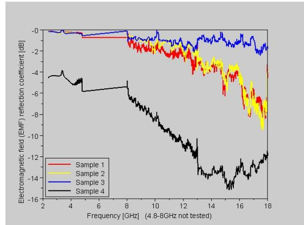
**Figure 4.** Characteristics of electromagnetic field (EMF) reflection coefficient of textile-polymeric shields.
