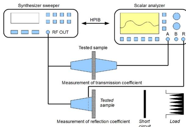
**Figure 2.** Block diagram of a measurement stand for the determination of EMF transmission and reflection.
