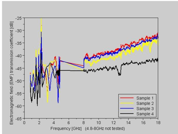
**Figure 3.** Characteristics of the electromagnetic field (EMF) transmission coefficient of textile-polymeric shields.
