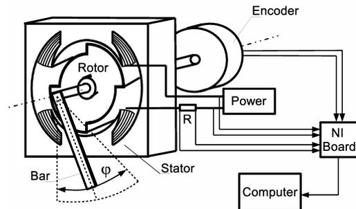
Figure 2: The measurement diagram of the reluctance motor parameters
