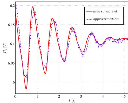
Figure 4: The waveform of voltage oscillation of the stator windings
