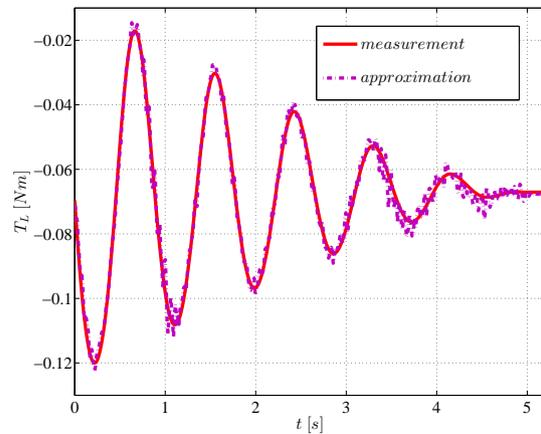
Figure 5: The oscillation of load torque in the mechanical equation
