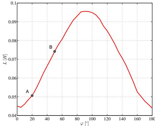
Figure 3: The inductance profile for the angle of rotation
