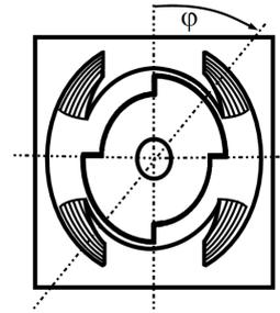
Figure 1: A general diagram of the reluctance motor
