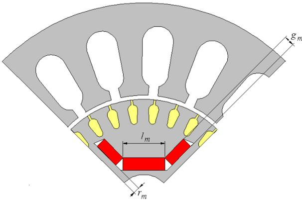
Figure 2: The LSPMSM structure
