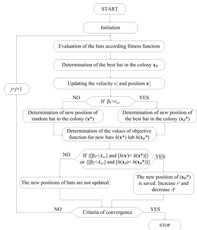
Figure 1: Flowchart of the bat algorithm
