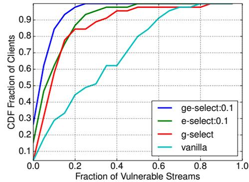
**Fig. 10.** Empirical CDF of the Fraction of Vulnerable Streams for e-select:  $\tau = 0.1$ , g-select, and g&e-select  $\tau = 0.1$  compared to Vanilla Tor for streams generated in Shadow simulations.
