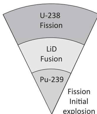
**Fig. 5.** 3F type hydrogen bomb.
