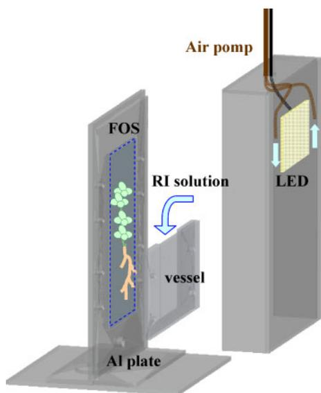
Fig. 2. Assembly of a plant sample container. The root of the sample plant was set in a culture vessel containing  $^{32}\text{P}$ . The vessel covered with light shield was placed as close as possible to the surface of FOS.
