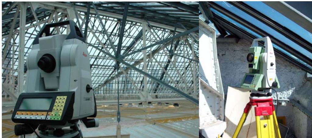
Fig. 1. Total stations TDA5005 (left) and TCRP1201+ (right) on the test object
