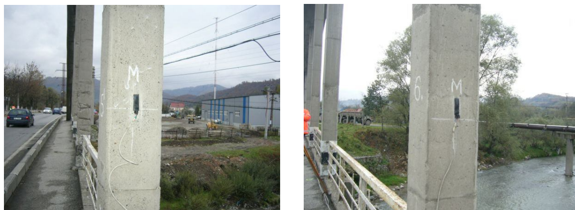
Figure 4. Electro-resistive transducers placed on the concrete hangers
