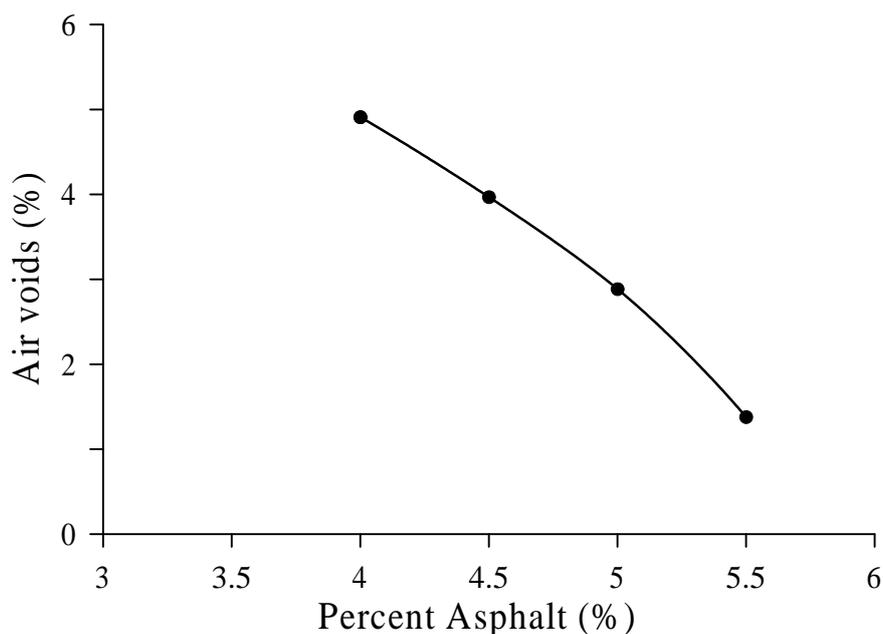
**Figure 4.** Air voids versus percent binder for the aggregate with dense gradation
