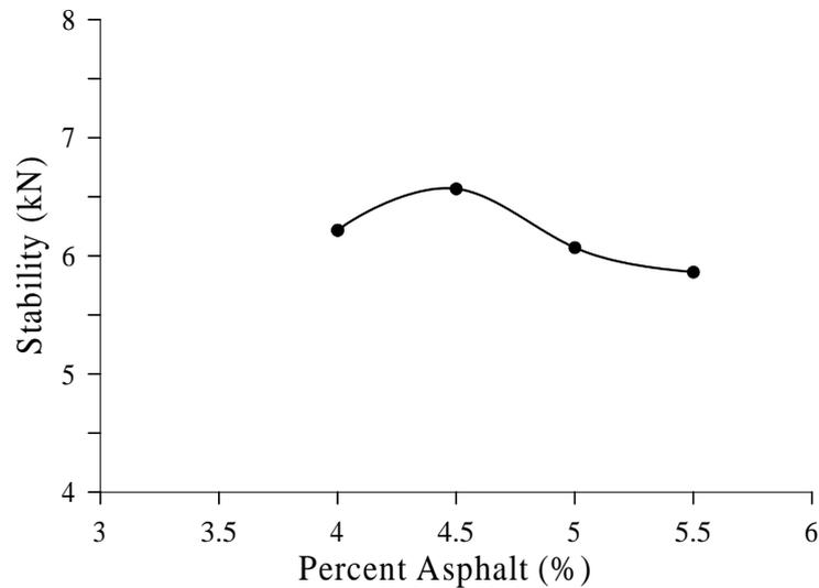
**Figure 9.** Stability versus percent binder in open graded mix (max grain size 9.5 mm)
