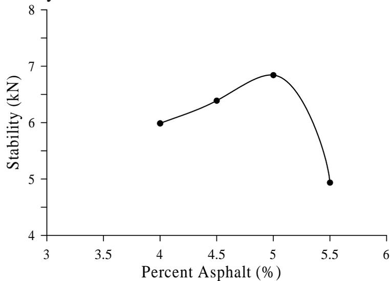
**Figure 7.** Stability versus percent binder in open graded mix (max grain size 19 mm)
